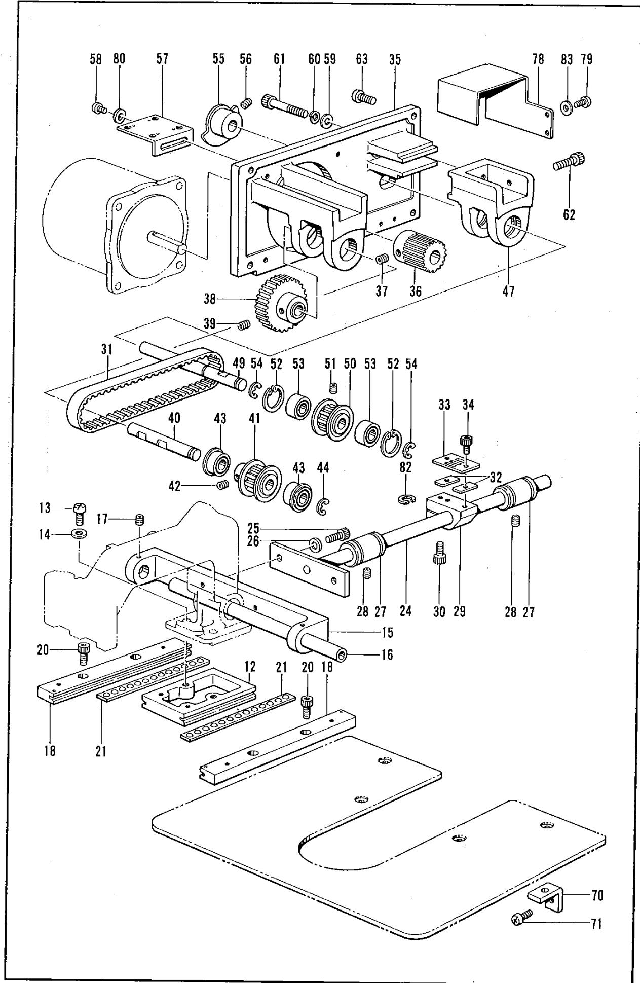
D3. 送り関係 /Feed mechanism /Transportvorrichtung /
