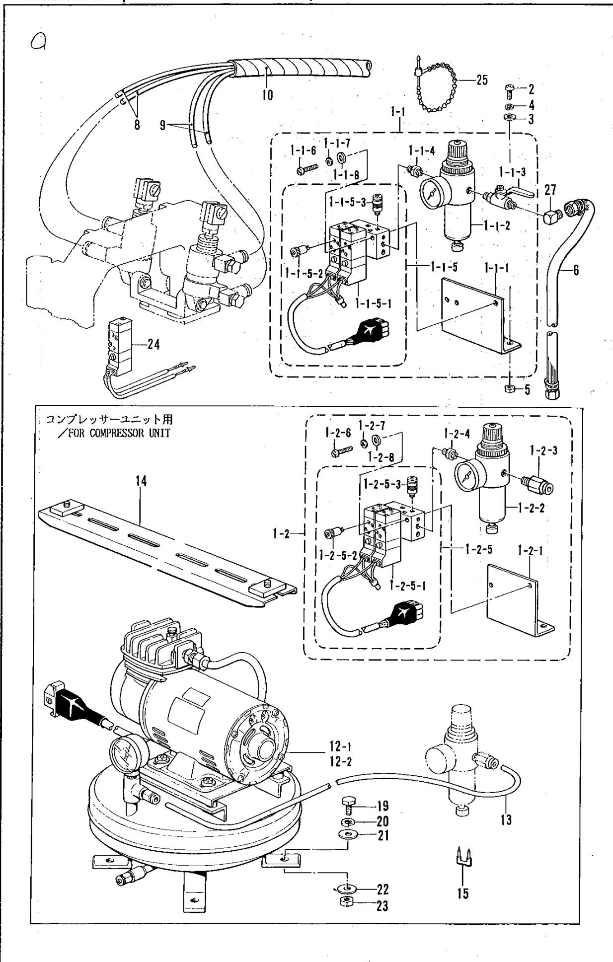
S. 空圧関係/Air pressure mechanism/Luftdruck/
