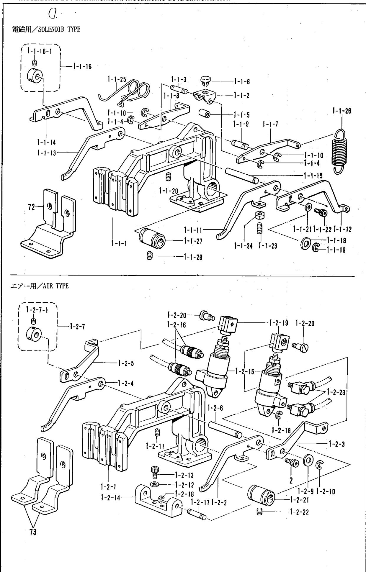
D1. 送り関係/Feed mechanism/Transportvorrichtung/
